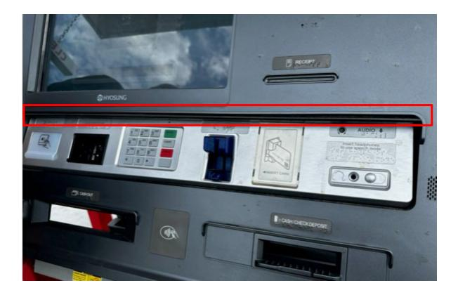
A false trim piece was applied to the front of the machine. The colors blended very well with the machine. The false trim was covering a built-in light on the machine.
