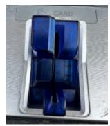
To the normal eye, a credit union member would not know that a skimming device resides inside the card reader. Cards inserted into the machine may have felt "tight" being inserted into the machine but otherwise unnoticeable. Upon closer examination, you can see a thin piece of metal in the machine which is the internal skimmer. The device is inserted into the machine just as a normal debit card but is
